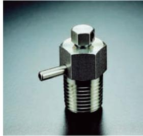
D-Pro VBV Series Bleed Valves are designed to vent the signal line pressure to atmosphere before an instrument is removed and to assist in calibration of control devices. These are for use on instrumentation devices such as gauge root valves and multi-valve manifolds. Optional barbed vent tube enables containment of fluid vented. The VBV Series are also ideal in bleeding hydraulic systems.
